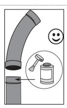
• If the inlet is installed upwards and the pipe runs straight up for 3 m or more, add two 22.5° elbows close to the inlet iFlex to keep the flexible hose slows down during its extraction.
