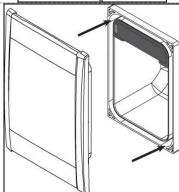
• Open the inlet door and fix the 4 screws supplied with it.
