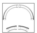
When it is possible to try to avoid the installation of 90 ° bends close together. We recommend always installing at least one meter of pipe between a 90 ° bend and the next.
